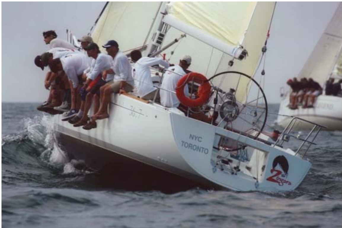
Sighting the side to side bend of the mast while sailing upwind in “race mode” Note that you can use the windward surface of the boom as a straight edge.
